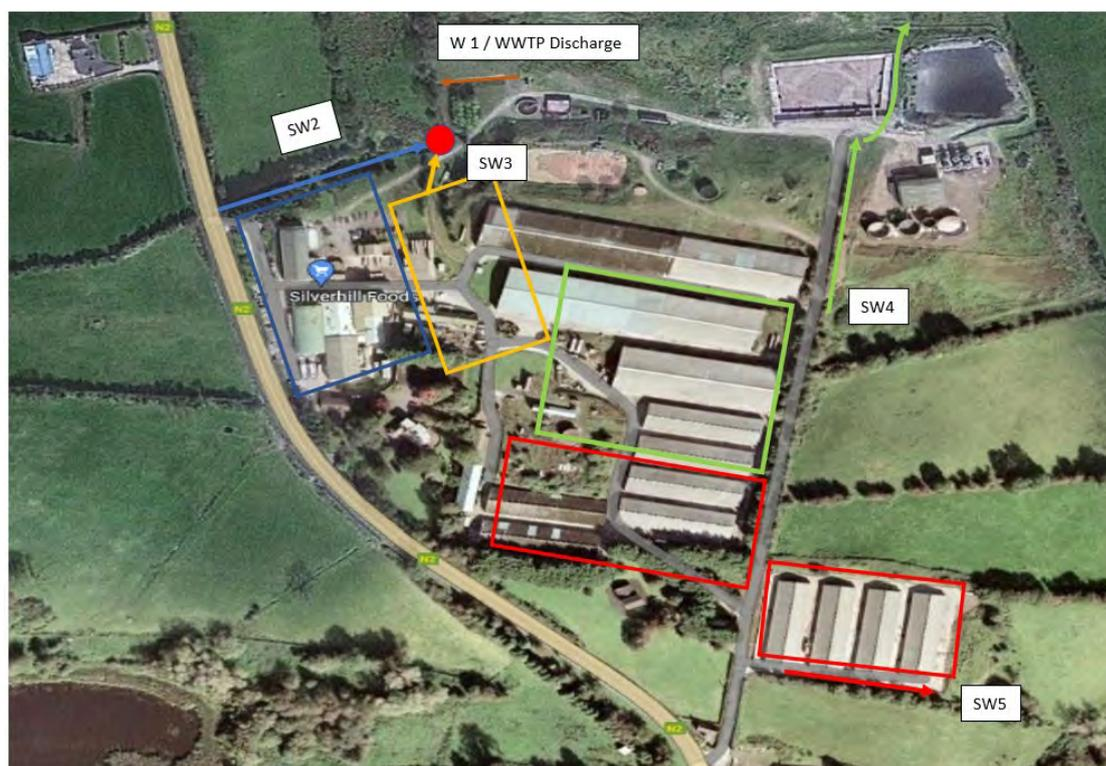
**Figure 7-2: Onsite Surface Water Drainage Map and IED licence monitoring points**
