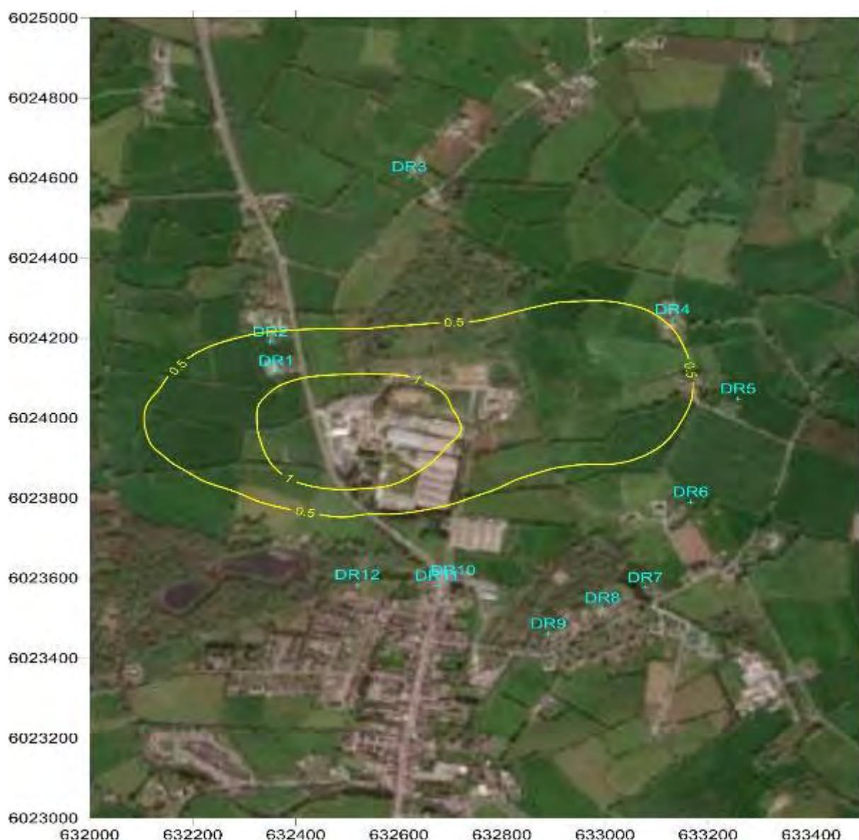
Figure 8-4 The ground level concentrations of odour predicted for cooking sources in the vicinity of the Silver Hill Foods Facility
